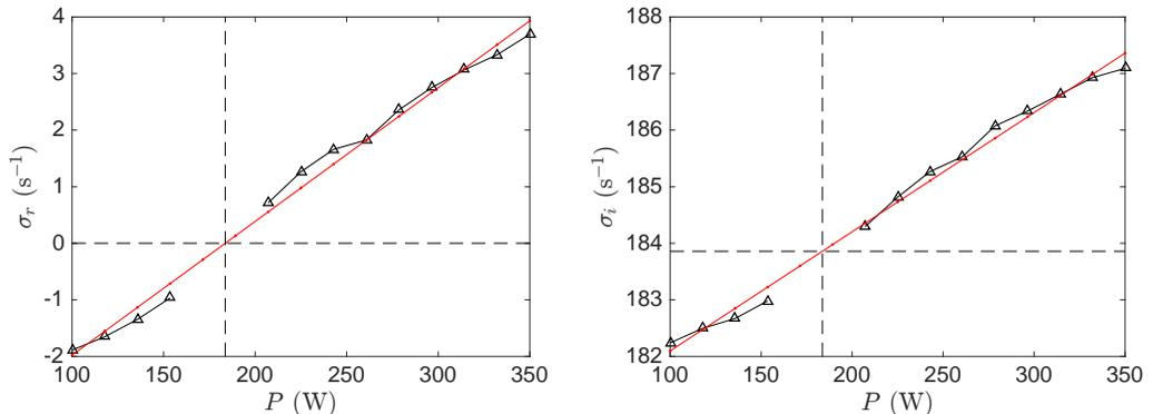
FIGURE 4. Linear stability characteristics for baseline case as a function of the primary heater power: (a) growth/decay rate,  $\sigma_r$ ; (b) frequency,  $\sigma_i$ . Experimental data (symbols) and linear fit (red line).
