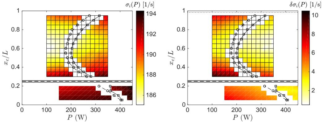
FIGURE 9. (a) Frequency and (b) frequency shift experimentally obtained as a function of power supplied to the heater and position of the drag device. Forward path critical powers (squares) and backward path critical powers (circles).
