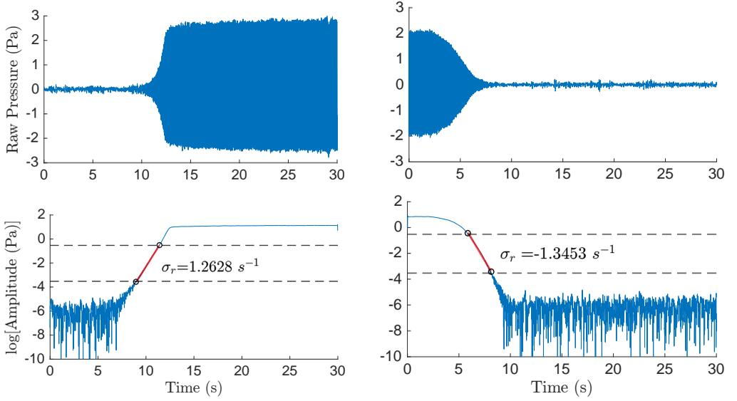
FIGURE 3. Top: Transient pressure signals obtained by applying step changes to the heater power input. (a) Growth, from  $P_H - \epsilon$  to  $P = 223 \text{ W}$ . (b) Decay, from  $P_f + \epsilon$  to  $P = 140 \text{ W}$ . Bottom: Amplitude of the filtered pressure signals obtained from the Hilbert transform. The linear growth (c) and linear decay (d) regions are represented by the red lines fitted between the noise floor and the point where nonlinear effects become important.
