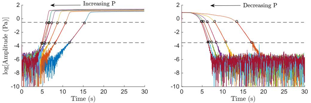
FIGURE 6. (a) Growth rates and (b) decay rates,  $\sigma_{r,c}$ , obtained with the control drag device positioned at  $x_c/L = 0.4$ . Each curve represents the amplitude response for a different departure size above or below the Hopf or fold point.
