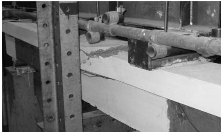
**Fig. 8–Flexural failure of F/295/LP1/3.3.**
