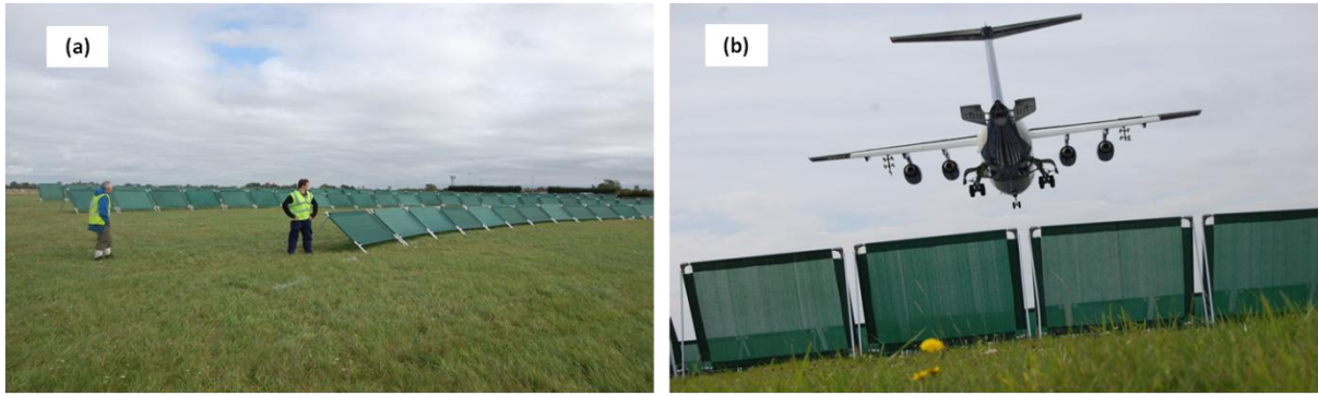
Figure 6.34. (a) Array showing three rows of baffles (in erect position) at Cranfield airport (September, 2011). (b) View from the last row of baffles during a landing routine during the field trials.
