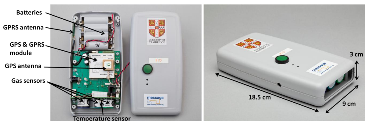
Figure 3.6. Mobile sensor node (type C) incorporating three electrochemical sensors (for CO, NO and NO 2 in this case). Components (GPS/GPRS module, batteries etc.) are identified in the left panel. For clarity, the unit is shown without its protective wire mesh, which, during operation, is located in front of the sensors.
