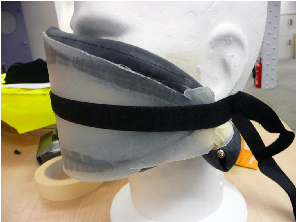
Picture 7.5 An initial sketch model to test mask potential sealing principle
