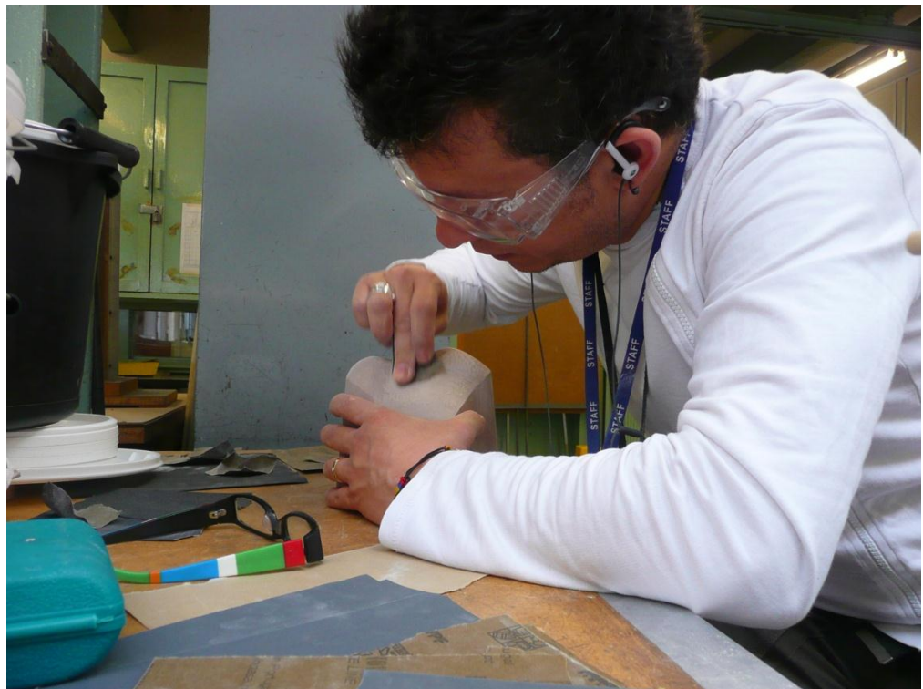
Picture 7.8 Designer finishing a CNC machined mould for the mask prototype
