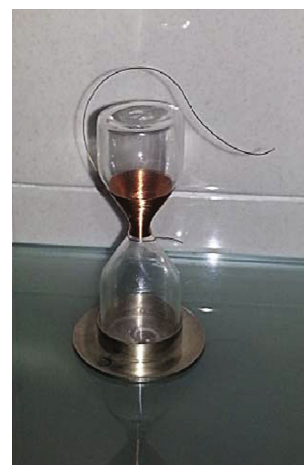
Fig. 5 The magnetic bottle with conical solenoid used in the experiments
