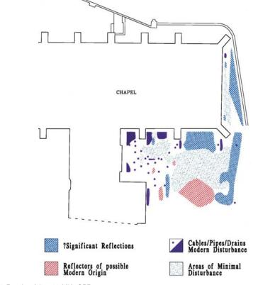
Fig. 7. Results of the 500-MHz GPR survey.
